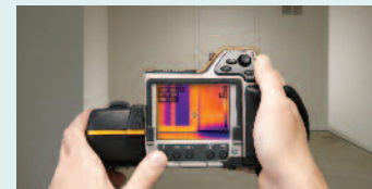
Infrared cameras quickly locate moisture related problems
